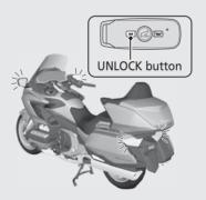
If you press the UNLOCK button, but nobody opens any of the compartments within about 30 seconds or about 30 seconds have passed after an opened compartment is closed, the compartments automatically will relock (Turn signals blinks once).
