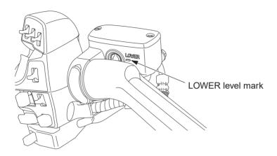
Check that the fluid level is above the LOWER level mark. If the fluid level is below the LOWER level mark, it indicates fluid leakage. See your dealer for repair.
