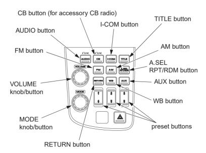
The CB lever and button function when the Honda accessory CB radio is installed. For CB operating instructions, refer to the accessory manual.
