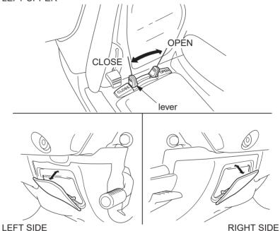
You can adjust the foot warmer ventilation louvers with the lever to control and direct the flow of warm air.
