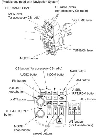
The CB lever and button function when the Honda accessory CB radio is installed. For CB operating instructions, refer to the accessory manual.
