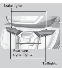
The brake lights, taillights and rear turn signal lights use several LEDs. If there is a LED which is not turned on, see your dealer for servicing.
