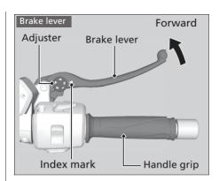
After adjustment, check that the lever operates correctly before riding.
