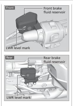
If the brake fluid level in either reservoir is below the LWR mark or the brake lever and pedal freeplay becomes excessive, inspect the brake pads for wear. If the brake pads are not worn, you most likely have a leak. Have your motorcycle inspected by your dealer.
