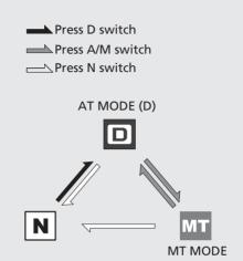
**Neutral (N):** Neutral is selected automatically when you turn the ignition switch to ON.
