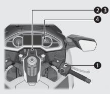
**5** Press the start button with the throttle completely closed.
