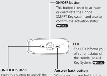
When pressing and holding the button with the electrical system off, your motorcycle informs you of its location by flashing the turn signal lights and sounding the
