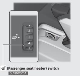
Turn to adjust the passenger seat heater level.
