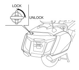
The saddlebags can be locked and unlocked with the ignition key.
