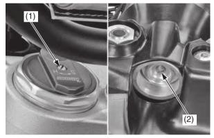
(1) compression damping adjuster(2) rebound damping adjuster
