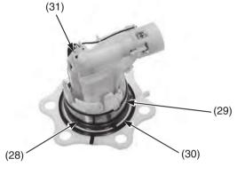
(28) O-ring (new) (29) dust seal (30) collar(31) fuel pump unit
