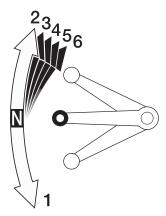
Your CRF has 6 forward gears in a one-down, fiveup shift pattern.
