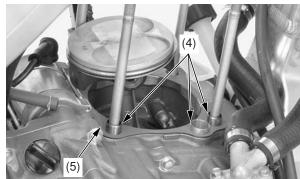
(4) dowel pins(5) cylinder gasket
