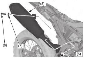
(5) right muffler mounting A bolt(6) right muffler mounting B bolt(7) washer(8) right muffler
