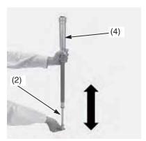
(2) fork damper piston rod (4) fork damper assembly
