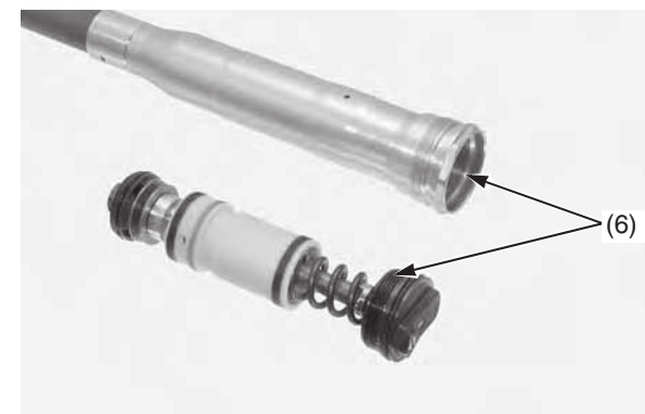
(6) fork bolt and fork damper assembly threads
