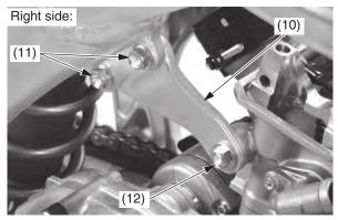
(9) left cylinder head hanger plate(10) right cylinder head hanger plate(11) cylinder head hanger plate bolts
