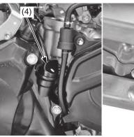
(4) engine oil fill cap/dipstick(5) engine oil drain bolt(6) O-ring (new)
