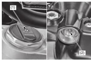
(1) compression damping adjuster(2) rebound damping adjuster
