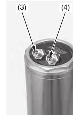
(3) inner chamber air valve (4) outer chamber air valve (5) balance chamber air valve (6) balance chamber air valve center
