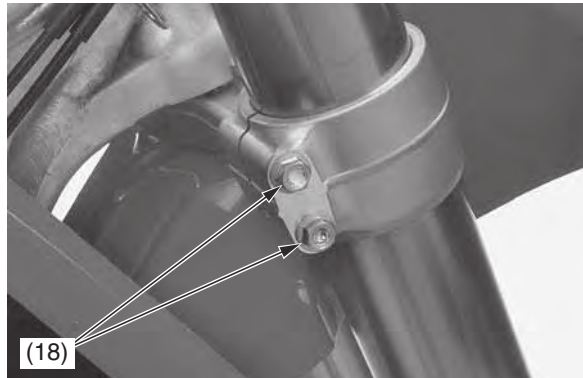
(18) fork bridge lower pinch bolts
