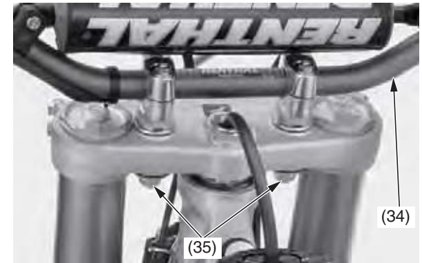
(34) handlebar (35) mounting rubbers, washers and handlebar lower holder nuts
