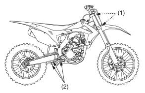
(1) steering head bearings(2) suspension pivot points
