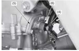
(4) tensioner stopper(5) cam chain tensioner lifter(6) handle
