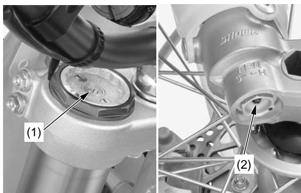
(1) compression damping adjuster (2) rebound damping adjuster
