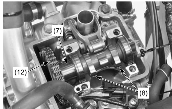
(7) cam shaft (8) intake cam lobes (12) cam chain
