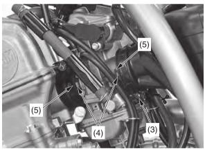
(2) insulator band screw(3) connecting tube clamp screw(4) tabs(5) grooves
