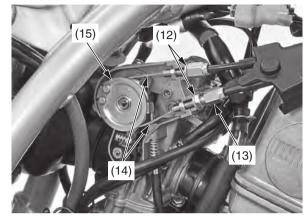
(12) lock nuts (13) adjuster (14) throttle cables(15) throttle drum
