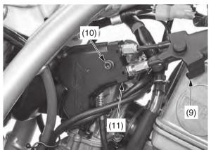
(9) dust cover(10) throttle drum cover bolt(11) throttle drum cover
