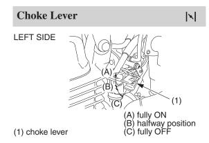
The choke lever (1) is used for starting the engine (page 29). The choke increases the percentage of fuel in the fuel/air mixture delivered to the engine.
