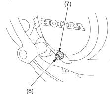
(7) clutch lock nut (8) clutch adjuster
