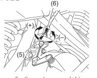
(5) lower adjusting nut(6) lower lock nut
