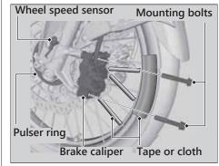
**3.** On the left side, remove the mounting bolts and remove the brake caliper.
