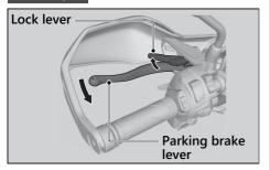
Place your motorcycle on a firm, level surface. Stop the engine and push your motorcycle while set the parking brake to check the efficacy of the parking brake.
