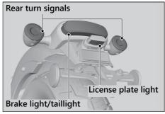
The brake light, taillight, rear turn signals and license plate light use several LEDs. If there is an LED which is not turned on, see your dealer for servicing.
