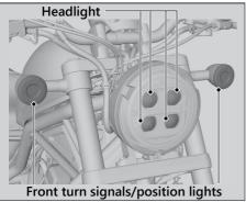
The headlight and front turn signals/position lights use several LEDs.
