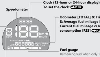
Odometer [TOTAL] & Tripmeter [TRIP A/B] & Average fuel mileage [AVG A/B] & Current fuel mileage & Reserve fuel consumption [RES] P.24
