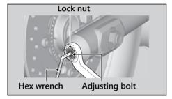
**6.** Tighten the rear axle nut.
