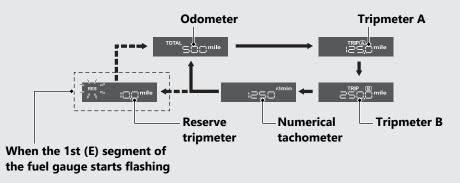
When the 1st (E) segment of the fuel gauge starts flashing, the odometer, tripmeters or numerical tachometer switches to the reserve tripmeter.
