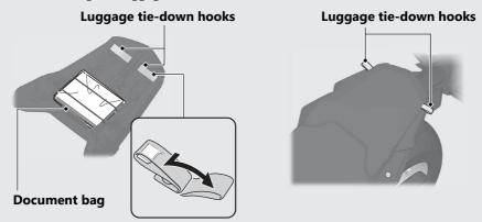
Never use the tie-down hooks to tow or lift the vehicle.
