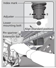
Attempting to adjust directly from 1 to 9 or 9 to 1 may damage the shock absorber.
