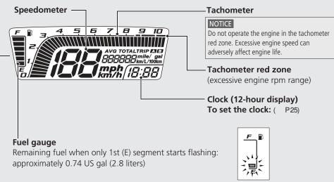
If the fuel gauge indicators repeat flashing or turned off: ( P91)
