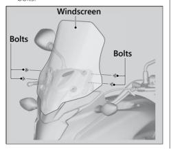
**2.** Install the right and left bolts to the low position holes or high position holes.
