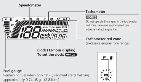
If the fuel gauge indicator flash sequentially or turned off: CR91
