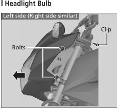
**1.** Remove the bolts and clip (2 P. 50) on both sides and pull the headlight assembly forward.
