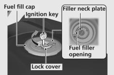
Do not fill with fuel above the filler neck plate. **Fuel type:** Unleaded gasoline only **Recommended fuel octane number:** Pump Octane Number (PON) 86 or higher.
