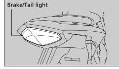
The brake and tail light uses several LEDs. If there is a LED which is not turned on, see your dealer for servicing.
