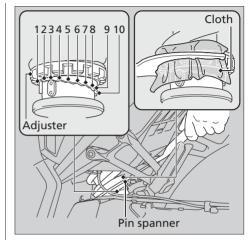
Attempting to adjust directly from 1 to 10 or 10 to 1 may damage the shock absorber.
