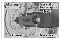
4. Turn both adjusting bolts an equal number of turns until the correct drive chain slack is obtained. Turn the adjusting bolts counterclockwise to tighten the chain, or clockwise to provided more slack. Adjust the chain slack at a point midway between the drive sprocket and the driven sprocket.
