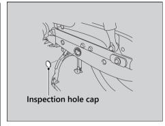
**3.** Remove the inspection hole cap.
